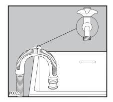
In a sink drain pipe branch. This branch must be above the trap so that the bend is at least 60 cm above the ground.
