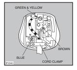
The wire coloured green and yellow must be connected to the terminal marked with the letter «E» or by the earth symbol  $\frac{\bot}{}$  or coloured green and yellow.
