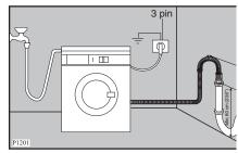
An additional drain hose and joining piece is available from your local Service Force Centre. The joining piece must have an internal diameter of 18 mm.
