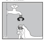
Set the hose correctly by loosening the ring nut. After positioning the inlet hose, be sure to tighten the ring nut again to prevent leaks.
