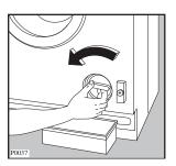
Unscrew and remove the filter.
