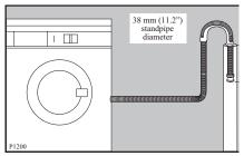
When discharging into a standpipe ensure that the top of the standpipe is no more than 90 cm (35.4") and no less than 60 cm (23.6") above floor
