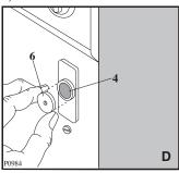
right, invert the position of the plates (7), the magnet (4) and the plate (5) (Fig. B and the hinges (1) as previously described.
