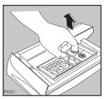
Detergent can also eventually accumulate inside the drawer recess: clean it with an old toothbrush. Refit the drawer after cleaning.
